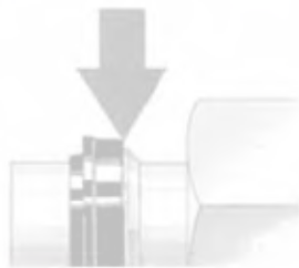
Fig. T50 — Ferrule cocked on tube
